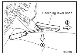
2. Remove the seat cushion front finisher and seat cushion outer finisher.
