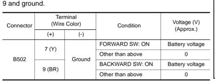
Check voltage between seat control unit connector B502 terminals 7,
