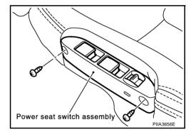
3. Remove the power seat switch assembly.
